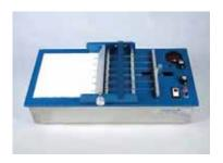
TLC Autospotter™ is a semi-automated device used to apply up to 18 samples on a TLC plate at a time. The unit has been designed for use TLC syringes with blunt Teflon tipped needles. These special needles minimize sample "creep back" and enhance reproducibility. The syringes also feature Teflon plunger tips to help eliminate the problem of metalto-glass contamination. Syringes are available in 10, 25, 50, 100 and 250µL volumes.
